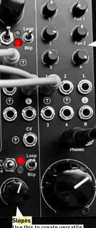
Use this to create versatile LFOs, envelopes, clocks and pulses. It's very loosely based on the Serge Voltage Controlled Slope circuit.
